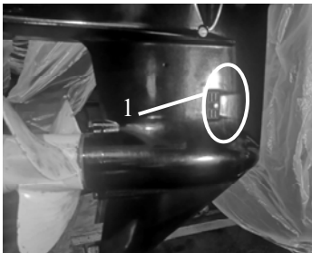
1. Inlet of cooling water channel
